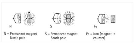
The counter is actuated by a magnetic field. With suitable magnets it is possible to achieve actuating distances of up to 50 mm. The direction of approach of the actuating magnet is not critical. When choosing a counter, it is important to observe the correct polarity of the actuator (see Figure).
